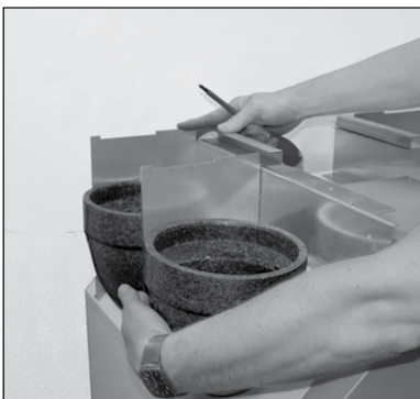
4. Attach the mounting to the U-profile
