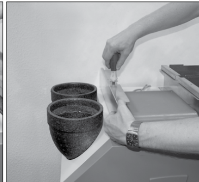
3. Locate U-profile and screw onto the CA 350
